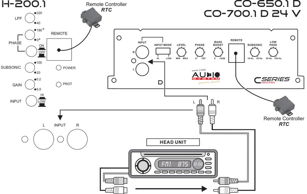
The **H/C SERIES** amplifier offers RCA-Inputs, which are connected through cinch cables with the preamplifier-outputs of the head unit. If the head unit (OEM-RADIO) has no RCA-Output, than it is possible to connect the speaker output direct to RCA/Cinch-Input of the amplifier.
