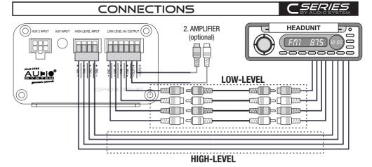
7. Pre-Out: The amplifier has a 2-channel pre-out to connect further amplifiers.
