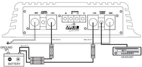
**1. Battery disconnection**: First, disconnect the power supply of the vehicle by removing the ground cable of the battery.
