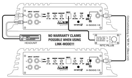
The IH-5000.1 D amplifiers offers RCA-inputs, which are connected by RCA cinh-cables to the preamplifier outputs of the headunit.
