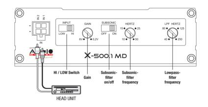
The X SERIES amplifiers have RCA inputs, which are connected by RCA cables to the preamp outputs of the head unit. If this is not possible (usually in an original radio, OEM) the speaker outputs of the car radio can be connected directly to the RCA / Cinch inputs of the amplifier. In this case, the Input Mode must be switched to "HI". It is important that the gain potentiometer is first set to minimum and turned up carefully when handling.
